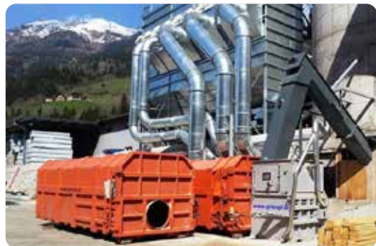
Disposal plant for wooden chips
